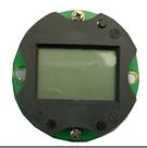
EST4300-A circuit board, available for small capacitance sensor, transmits differential capacitance signals to two-wire 4--20 mA with stable and reliable performance. Compatible with ROSEMOUNT 's 275/375 communication interface and conforming to the HART protocol, EST4300-A can perform temperature compensation at two pressure points and three temperature points.
