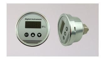
ESG102 line digital pressure gauge is full electronic structure which adopts oil-filled diaphragm piezoresistive sensor; the output signal with high precision, low temperature drift has been treated by amplifier amplification process, and then inputted into the high precision A/D converter heading for digital signals, and finally been displayed via LED display to indicate the actual pressure performance/value.
