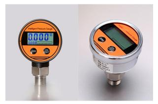
ESG103 line digital pressure gauge is full electronic structure and battery based power supply model, ESG103 adopts oil-filled diaphragm piezoresistive sensor for a relative high accuracy and good stability; the output signal with high precision, low temperature drift has been treated by amplifier amplification process, and then inputted into the high precision A/D converter heading for digital signals, and finally been displayed via LED display to indicate the actual pressure performance/value.
